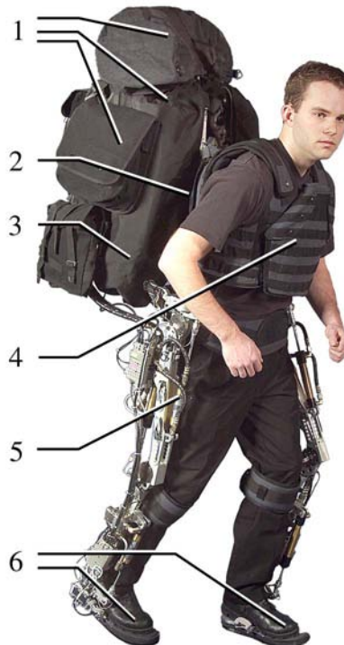
Fig. 1 Berkeley Lower Extremity Exoskeleton (BLEEX) and pilot Ryan Steger. 1: Load occupies the upper portion of the backpack and around the Power Unit; 2: Rigid connection of the BLEEX spine to the pilot's vest; 3: Power unit and central computer occupies the lower portion of the backpack; 4: Semi-rigid vest connecting BLEEX to the pilot; 5: One of the hydraulic actuators; 6: Rigid connection of the BLEEX feet to the pilot's boots. More photographs can be found at http://bleex.me.berkeley.edu
