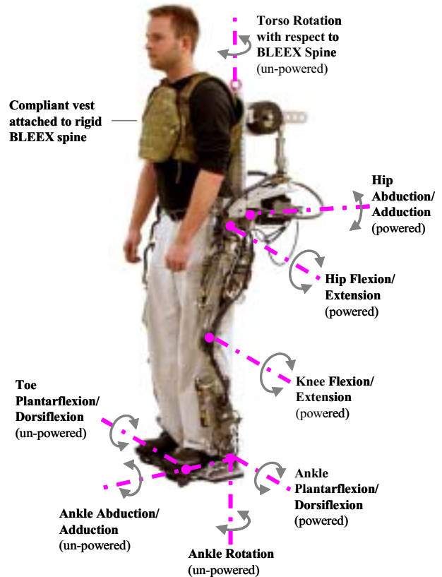
Fig. 2. BLEEX mechanical structure and degrees of freedom.
