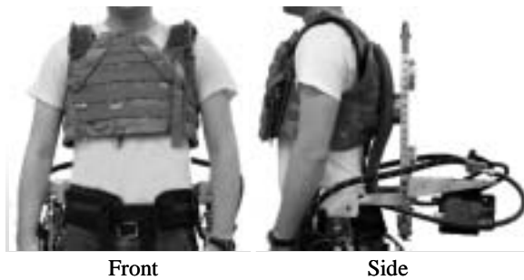
Fig. 3. The pilot vests in this figure and in Figure 1 are designed to uniformly distribute the BLEEX-pilot force on the pilot's upper body (note that the BLEEX power supply is not attached in the "side" image).
