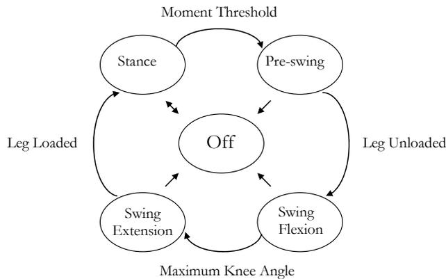
Fig. 10 State-machine diagram for the knee controller.
