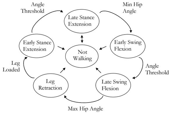
Fig. 7 State-machine diagram for the hip controller.
