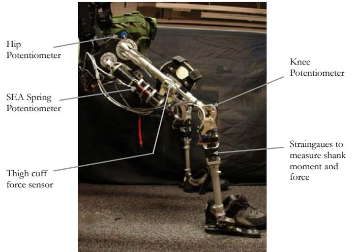
Fig 4. Sensors placed on the exoskeleton leg.
