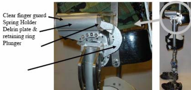
Fig. 15 Extension spring assembly mounted on the exoskeleton.
