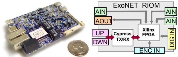
Fig. 9 ExoNET RIOM photo and schematic. Each RIOM provides for 3 analog inputs (AIN), 1 analog output (AOUT), 6 digital inputs (DIG IN), 1 quadrature encoder input (ENC IN), and 2 network communication ports (UP and DWN). Two integrated circuits handle processing (Xilinx Inc.) and network communication (Cypress Semiconductor Inc.) respectively.
