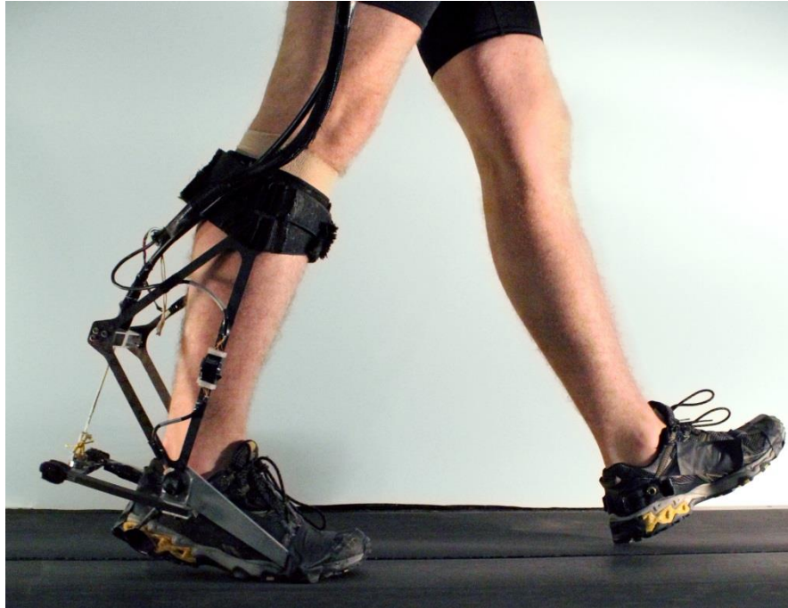
Fig. S3. Photograph of the ankle exoskeleton used in the main experiment.
