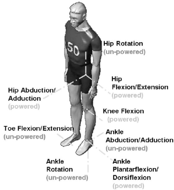
**Figure 2.** Exoskeleton d.o.f.
